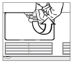
Open the access panel, located on the lower left corner of the machine, using the yellow tool supplied with the machine.
