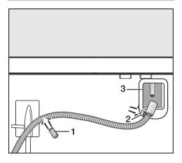
Unclip the drain hose from the clamps 1 and 2, and pull it off the holder, 3.
