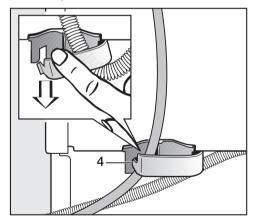
■ The lower clamps, 4, can be opened to install the drain hose or to feed the power cable through.
