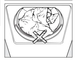
■ Before closing the door make sure the fluff filter is correctly positioned.
