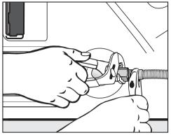
■ Secure the flexible metal gas line connector to the adapter.
