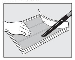
■ Wipe the lint off the filter with your hand (do not use any sharp objects!) or use a vacuum cleaner with the supplied vacuum cleaner nozzle.
