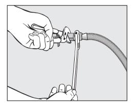
Using two adjustable wrenches tighten all connections.
