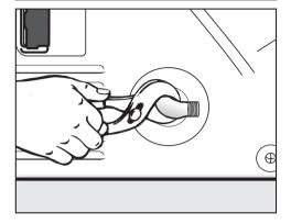
■ Install a female <sup>3</sup>/<sub>8</sub>" NPT elbow at the end of the dryer's gas connection.
