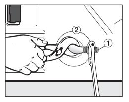
Install a <sup>3</sup>/<sub>8</sub>" flare union adapter, ①, to the female elbow, ②.
