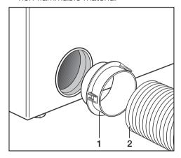
■ Install the connector, **1**, with the exhaust hose or pipe, **2**, to the dryer.
