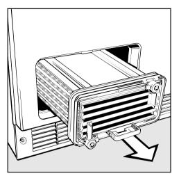
■ Pull out the heat exchanger.
