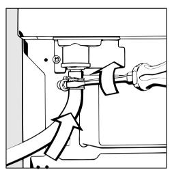
Push the drain hose onto the drain outlet. Make sure that the hose is firmly secured by the hose clamp and not kinked.
