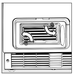
■ Turn both levers on the heat exchanger so that they are vertical
