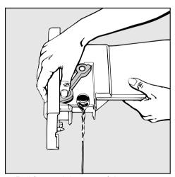
Pull forward the cap of the spout as indicated by the arrow and hold open while emptying the container.
