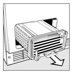
■ Pull out the heat exchanger
