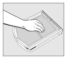
Use your fingers to remove the fluff from the surface of the filter. Remove any fluff from the hollow part of the door holder. A cleaning brush is available as an optional extra from your Miele dealer or the Miele Spare Parts Department.
