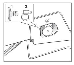
Remove the following from the back of the dryer at the bottom: Adapter 1 and hose clip 3 behind it.
