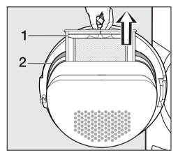
Open the door and pull the fluff filter
