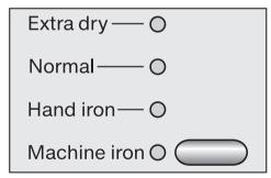
Press the drying level button repeatedly until the indicator for the drying level you want lights up (for almost all programmes).
