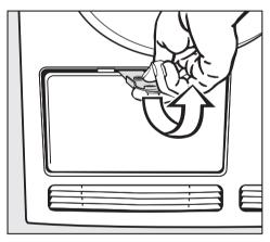
Now remove the panel by pulling it diagonally upwards and place it to one side.
