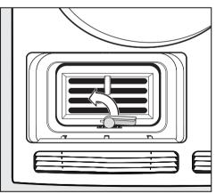
Turn the lever on the condenser unit upwards to the vertical position so that the hook on the lever is no longer in the groove at the bottom of the condenser unit housing.
