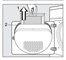
Open the door and remove the lint filter, 1, by gently lifting it upwards.
