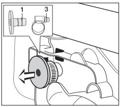
Remove the accessories from the top rear of the dryer: Connector 1 and the hose clamp 3 behind it.
