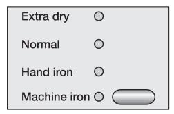
Press the Drying level button repeatedly until the indicator light for the drying level you want lights up.
