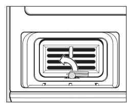
Turn the lever on the condenser unit upwards to the vertical position so that the hook on the lever is no longer in the groove at the bottom of the condenser unit housing.
