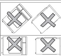
If the tumble dryer has not been transported as described, then it must be left to stand for at least 1 hour <u>before</u> it is connected to the electricity supply. Otherwise the heat pump can be damaged.
