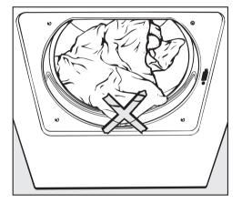
When closing the door make sure items of laundry cannot be trapped by the door, as this will cause damage to the laundry.
