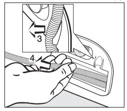
■ Then pull the drain hose completely out of the dryer towards the left (4) (See illustration).
