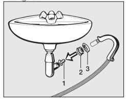
If this nut has a flat disc sealing it you should take the disc out first.
