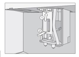
■ Push the catch upwards ①, grasp the dispensing unit by the handle and pull it out towards the front ②.
