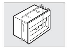
■ If there is no sealing strip around the installation recess, stick the Miele sealing strip onto the unit from the back before putting it into the recess. The sealing strip is available from Miele.
