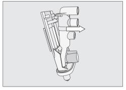
Hold the magnets at the side and pull forwards to release the unit.
