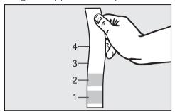
■ Dip the test strip into your tap water for about one second. Then shake off any excess water. The result will be visible after about one minute.
