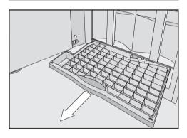
Open the front door and carefully remove the drip tray.
