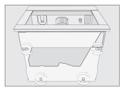
Unscrew the four feet on the underside of the unit by about 1/16" (2 mm) using the larger Allen wrench.
