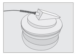
■ Use the cleaning brush to clean the milk pipework in the lid as well.
