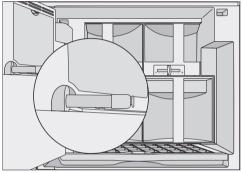
Once a month, lubricate the cap with the silicone grease provided.
