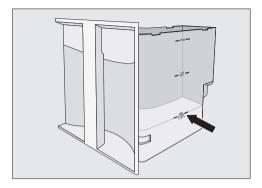
■ Fill the water tank with lukewarm water up to the ///\\ mark and stir the solution.
