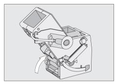
Push the coffee ejector of the brew unit into the correct position (see image).
