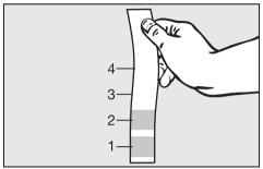
Dip the test strip in water for about one second. Then shake off any excess water. The result will be visible after about one minute.
