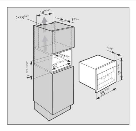
A combination with other built-in Miele appliances is possible. For combination installations, it is very important to install the unit with a protective base between the appliance and the unit (exception: installation with a built-in plate warmer).
