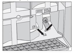
Carefully clean and dry the surface the water tank sits on, particularly the slots.
