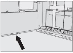
■ Remove this cup and clean it in the dishwasher or by hand using warm water and liquid dish soap.
