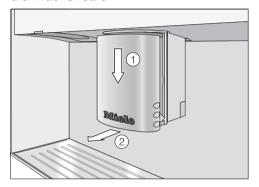
■ Pull the main dispenser all the way down ① and pull the cover forward to remove ②.
