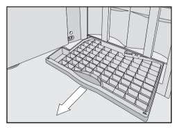
Open the appliance door and carefully remove the drip tray from the appliance.
