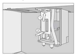
■ Push the snap-in clip slightly up ①, seize the grip of the dispensing unit and pull it out towards the front ②.
