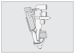
■ Release the dispenser by seizing it by the sides of the magnet and pulling it to the front.
