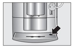
Replace the drip tray cover. Be sure the outer hole is located under the cappuccinatore.
