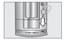
■ Remove the cappuccinatore from the steam and hot water spout by pulling it downwards.
