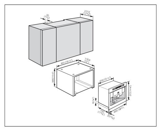
To install the CVA 2650 below a hanging cabinet a **CVUG 50** casing (optional accessory) is required.
