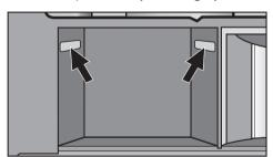
Clean the waster container niche. Be sure to clean the sensors, left and right, the sensors read if the waste container is inserted and if it needs to be emptied.
