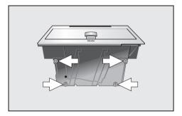
Push the appliance all the way back into the cabinet and center it. If necessary level the unit with the four height adjustable feet.
