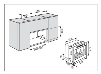
It can also be combined with other Miele built-in appliances. If the coffee machine is to be built in above another appliance, there must be a full-width, closed shelf between them (except when it is combined with a Miele built-in plate warming drawer).
