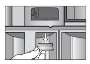
Pull the rubber connector downwards. Hold it by the edge to lever it downwards.
