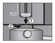
■ To make the froth press on the steam valve ① to connect the valve to the milk frother ②.
