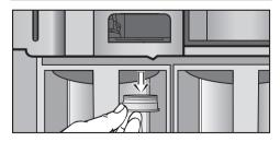
Pull the rubber connector downwards.
