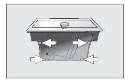
Check the height of the machine to make sure that it is sitting centrally in the niche and that it is level. If this is not the case, realign the 4 feet underneath the machine using the large allen key.
