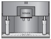
Set the descaling funnels under the hot water and froth dispensers. Set the funnel in the holes of the drip tray so the dispensed liquids are guided in the drip tray.
