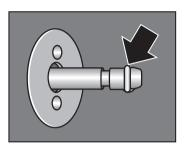
The part which connects the brew unit and the coffee outlet is located on the inside of the machine door.
