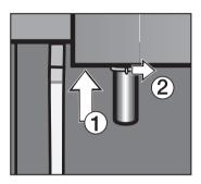
Place the Cappuccinatore in the machine from below ① and turn the cover above the spout in the direction of the arrow ②.
