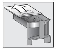
Push back the lid and fill the container with roasted coffee beans. Pull the lid forwards again, push the coffee bean container back into place and close the machine door.
