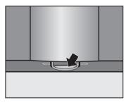
Also clean the small drip tray in the lower part of the inside of the door thoroughly.
