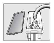
■ Open the lid and fill the container with cold drinking water to within about 1" (2 cm) of the top.
