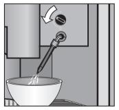
■ Place a 1 liter container below the steam nozzle and turn the steam selector counterclockwise.
