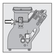
Check that the brew unit is in the basic position with the funnel slightly lifted and the socket in the vertical position (see illustration).
