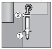
■ Push the sleeve onto the steam nozzle, ①, and tighten the screw, ②.
