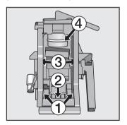
■ Lubricate the joints, ①, the axle, ②, the tracks, ③, and the gasket, ④, with silicon grease.
