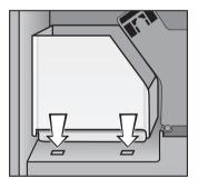
■ Push the waste unit back into place, positioning it over the notches.
