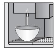
■ Place a large container (approximately 1 litre) under the steam spout and turn the steam control dial anti-clockwise.
