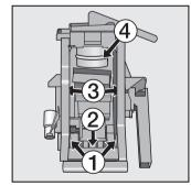
■ Clean the bolt ①, and smear a little silicone lubricant on it and on the joints ②.
