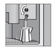
■ Move the jug in circles until a thick froth has built up, then lower the spout deeper into the milk to heat the rest
