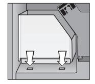
If the "Empty waste unit" message appears in the display window after you have just cleaned the unit out you will need to take it out of the machine and push it back into position again and then press the ENTER button. Otherwise the machine will get blocked. This is a safety feature to prevent the waste unit from overflowing. The machine counts the number of times coffee grounds are emptied into the waste unit. It automatically prompts you to empty it after a certain number of times.
