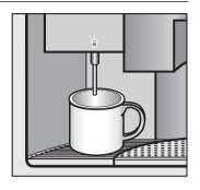
■ Press the hot water button 📵 until the cup is as full as required. Then release the hot water button 📵.
