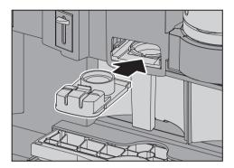
remove the capsule plate and replace it with the red descaling funnel.
