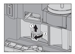
Insert the maintenance tool into brew unit ① from below and turn capsule hopper ② to the left to remove it.
