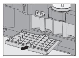
Open the front of the coffee machine. Remove the drip tray from the machine with care.
