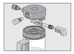
Reassemble the parts of the lid as shown.
