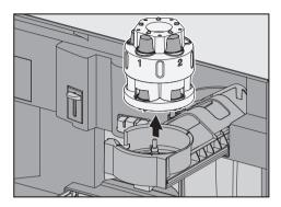
Open the front of the coffee machine. Pull the carousel runners out as far as possible and remove the capsule carousel.
