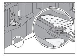
Also clean the small drip catcher in the lower part of the inside of the front of the machine thoroughly.
