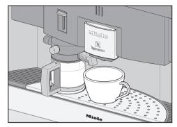
Place the cappuccinatore into the inset in the drip tray and place a cappuccino cup under the central spout.
