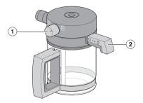
The cappucinatore must always be assembled correctly with value ① above the handle and spout ② at the side.
