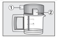
Above the handle on the cappuccinatore there is a valve ①, and a milk spout ② on the side.
