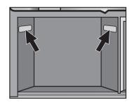
Clean the sensors, left and right, in the waste container niche. The sensors read if the waste container is inserted and if it needs to be emptied.
