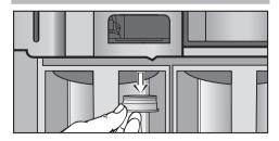
Pull the rubber connector down and out.
