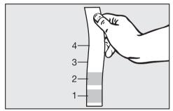
Place the test strip under your kitchen tap for a second and shake off any remaining water. The result is visible in about 1 minute.
