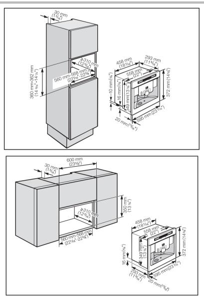
A combination with other Miele built in appliances is possible. If the machine is installed in combination with other appliances, it should be installed with a protective base between the appliance and the unit (exception: installation with a built-in plate warmer).
