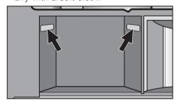
Clean the waste container niche. Be sure to clean the sensors, left and right, the sensors read if the waste container is inserted and if it needs to be emptied.
