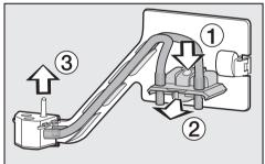
Do not pull the milk hoses off the retainers. This may cause the milk pipework to leak.
