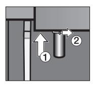
Push the froth dispenser into the machine from underneath, ①, and turn the cover above the spout to the right, ②.
