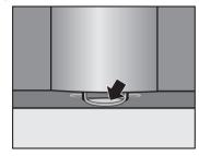
The lower part of the inner door has a drip tray. Clean the drip tray.
