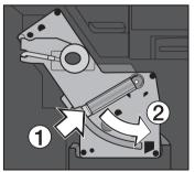
Press the light colored button on the brew unit handle, ①, and turn the handle to the right, ②.
