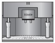
Set the descaling funnels under the coffee dispensers. Set the funnel in the holes of the drip tray so the dispensed liquids are guided in the drip tray.
