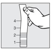
Dip the test strip in the water for 1 second and shake off any remaining water. The result is visible in about 1 minute.
