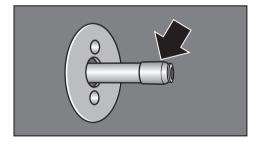
The part which connects the brew unit and the central spout is located on the inside of the machine door.
