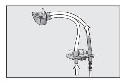
Push the brush into both milk pipes from below. Move the brush in and out of the pipes as far as it will go until there are no milk residues left in them.
