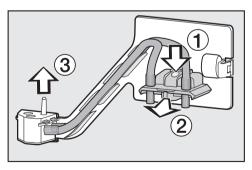
Press down on the small recess in the spout's holder (1) and pull the holder forwards and out (2). Loosen the milk pipework from its guides.
