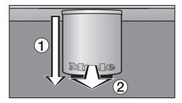
Pull the central spout down as far as it will go (①), and pull the cover to the spout forwards to remove it (②).
