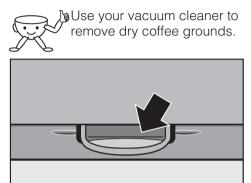
Also clean the small drip tray in the lower part of the inside of the front of the machine thoroughly.
