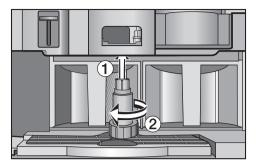
Using the special tool (supplied) as shown above, turn the capsule hopper to the left to remove it.
