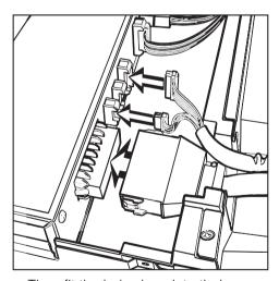
Then fit the hob plugs into their sockets. Push the cooker into the housing unit as far as the oven trim and align.
