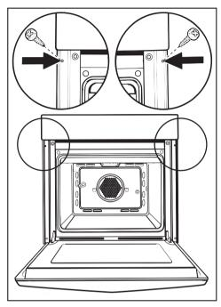
Then open the door and using two screws secure the oven to the side walls of the housing unit through the holes in the oven trim.
