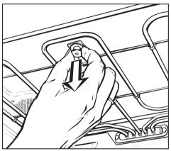
Pull down on the fixing knob for the element to release it.
