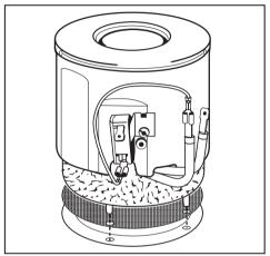
A catalyser can be built into the cooling system of the cooker or oven to filter fatty vapours and reduce food smells.
