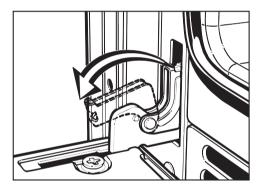
Before the door can be removed, the door hinges need to be locked so that they do not damage the door when it is taken out.
