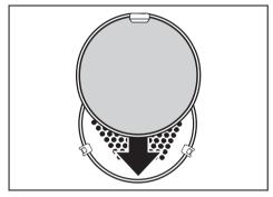
The droplets of fat caught up in the circulating air are deposited on the roasting filter. This helps to keep the oven and the area behind the interior back panel cleaner.
