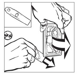
Press the lamp back into the sidewall of the oven and reinsert the cover.
