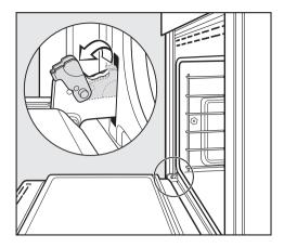
Prepare the doors for removal. Flip up the locking clamps on each door hinge.
