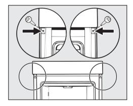
Open the oven door and using two screws secure it to the side walls of the housing unit through the holes in the oven trim.
