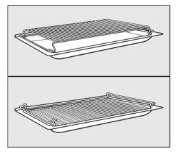
It can be used either way up to vary the height between it and the grill element, depending on the cooking function and type of food being cooked.
