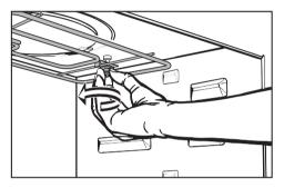
To lower the grill element loosen and then remove the nut.
