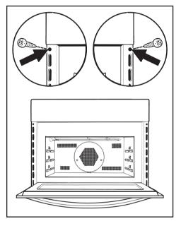
Open the oven door, and with two screws secure the oven to the side walls of the furniture unit through the holes in the oven trim.
