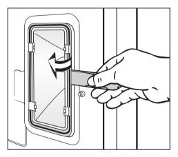
■ Use the lever to release the lamp cover from its frame.
