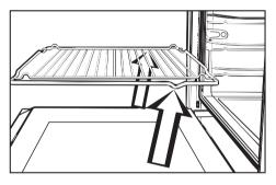
When pushing the tray, pan and rack back in, always ensure that the safety notches are at the rear of the oven (see illustration).
