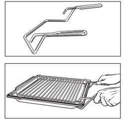
The handle makes it easier to take the baking tray, grill pan and rack out of the oven, or to put them into it.
