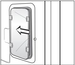
Push the glass cover back into the metal clamps with the cut out edge towards the rear.
