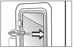
Replace it with a new one, making sure it goes into its socket horizontally.
