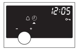
To **select a function**, turn the multi-function selector until **triangle** ▲ **is underneath the required symbol** in the display of the function you wish to make changes to.
