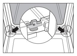
The oven door is connected to the oven by hinges.
