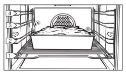
Place cakes in **rectangular tins** with the longer side across the width of the oven as shown, for optimum heat distribution and even results. Always use shelf level 1 for cakes in tins.
