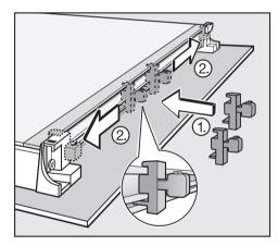
Lift the upper of the two middle panes up a little and refit the spacers to the panes. Then re-position them back next to the hinge guides.
