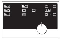
Turn the programme selector clockwise or anti-clockwise to the required oven function.
