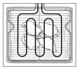
For grilling thin cuts and for browning food. The inner part of the upper heating element gets hot.
