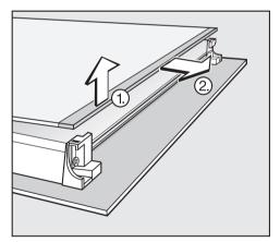
Carefully lift the inner pane up and out.
