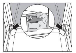
Before removing the door, the locking clamps on both hinges have to be released.
