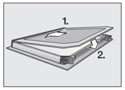
■ Push the inner pane into the plastic strip and place it in between the retainers
