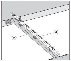
■ Insert the sealing strip ④ into the slots in the support bar ②.
