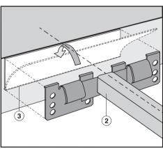
■ Position and attach the spring clips
