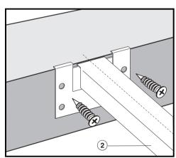
■ Place the supplied spring clips ① and the support bars ② at the marked positions as shown above, by laying them on the upper edge of the cut-out and then securing them with the ¹/₀" x 1" (3.5 x 25 mm) screws (supplied).
