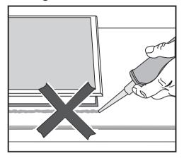
The appliance must not be permanently sealed into the countertop when installed. The sealing strip under the edge of the appliance provides a sufficient seal for the countertop.
