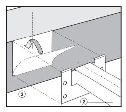
Position and attach the spring clips
