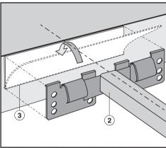
■ Position and attach the spring clips
