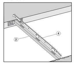
Insert the sealing strip 4 into the slots in the support bar 2.
