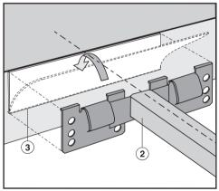
Position and attach the spring clips
