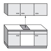
The minimum safety distance given by the hood manufacturer must be maintained between the fryer and the hood above it. See the installation instructions of the hood for these safety measurements.
