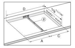
For the installation of **two appliances** the width of the countertop cut-out D is the sum of A and C.
