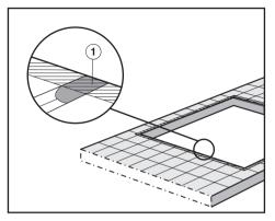
The appliance must not be permanently sealed into the countertop when installed. The sealing strip under the edge of the appliance provides a sufficient seal for the countertop.
