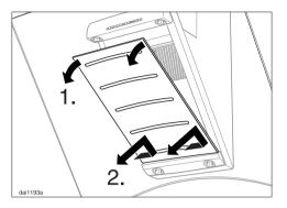
Pull the vapour plate down towards you at the top, push the bottom slightly to the right and pull forwards to remove (see illustration).
