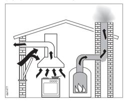
Ventilation can be maintained by air inlets which cannot be blocked, in windows, doors and outside wall vents, or by other technical measures, such as ensuring that the cooker hood can only be switched on when the heating appliance is switched off or vice versa. A ventilation brick alone is not generally sufficient to ensure safe ventilation.
