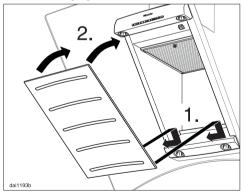
Hook the vapour plate into the bottom of the housing, push it slightly to the left and then raise it up towards the appliance and click it into position.
