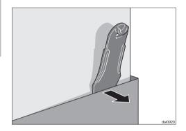
After loosening the fixing screws on the tower, push the lever between the tower and the extension piece to lever the tower out of its fixings.
