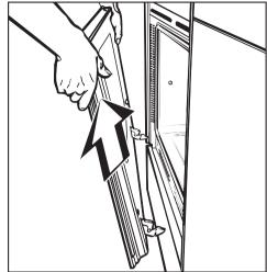
■ Lift up the door until the hinges disengage. Remove door.
