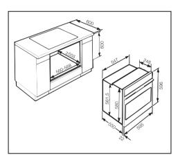
Push the cooker into the housing unit as far as the oven trim and align.
