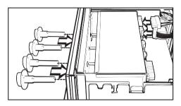
Insert the hob control knobs into the control facia.
