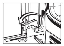
Flip down the locking clamps on each door hinge. This locks the hinges.
