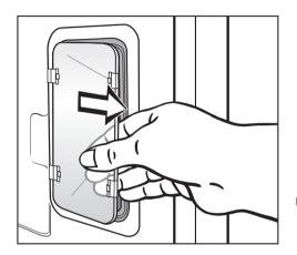
Pull the glass cover out of the rear metal brackets.
