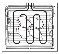
For grilling small quantities of thin cuts and for browning small dishes of food. The inner part of the grill element is switched on and glows red.
