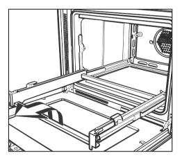
Remove the frame from the guide rails.
