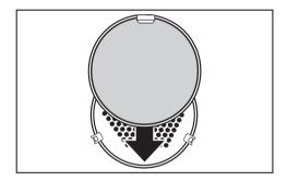
The droplets of fat caught up in the circulating air are deposited on the roasting filter. This helps to keep the oven and the area behind the interior back panel cleaner.
