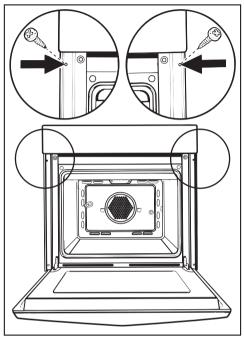
Open the oven door and using two screws secure the oven to the side walls of the housing unit through the holes in the oven trim.
