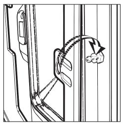
Lift the front locating hole on to the guide pin behind the collar.
