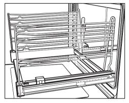
When pushing the baking trays, grill pan / oven tray or rack into the oven, make sure that the telescopic carriage is pushed completely in.
