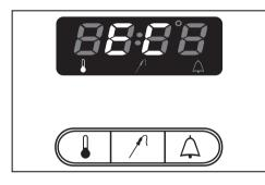
The letters "*EC*" in the display field indicate that the energy-save function is in operation.
