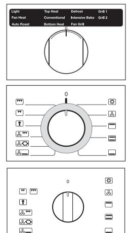
The function selector can be turned clockwise or anti-clockwise.
