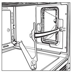
Put the runners or the guide rails of the telescopic frame back into place.
