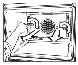
Loosen the screws in the back panel and take it out.
