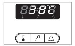
the actual core temperature appears in the oven display. N.B. The lowest temperature that can be displayed is 20°C, so this will also be shown until the roast probe registers 20°C.
