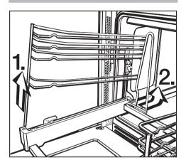
Pull out the telescopic carriage and remove the side runners.
