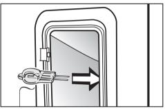
Pull the defective halogen lamp out and replace it with a new one, making sure it goes into its socket horizontally.
