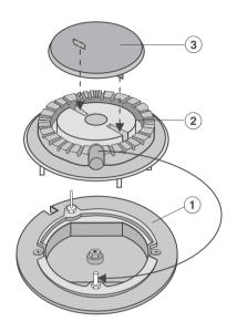
Be careful not to mix up the parts. Make sure that all the locating tabs and notches align exactly.
