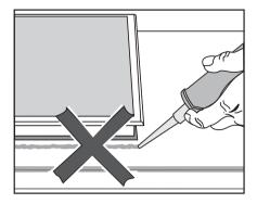
The sealing strip under the edge of the top part of the cooktop provides a sufficient seal for the worktop.
