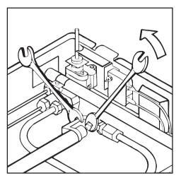
Changing the main jet, (does not apply to conversion to Natural Gas).
