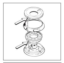
Important: The burner must be correctly fitted together before it is lit, otherwise the ignition device could be damaged.
