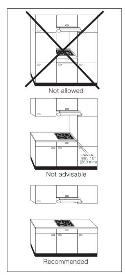
With kitchen cabinetry, the following minimum dimensions must be kept: – a distance of 10" (250 mm) from adjacent units if they are susceptible to heat, otherwise some form of insulation must be installed. – a distance of 30" (76 cm) between the cooktop and any wall cabinet installed above it.
