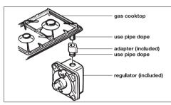
A straight thread adapter, from 1/2" ISO 7-1 to 1/2" NPT is included with the appliance.
