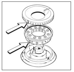
If, after several attempts the gas still does not burn, check whether the lug of the large burner cap is correctly positioned in the notch in the large burner cap base and whether the lug of the large burner cap base is correctly positioned in the notch in the burner base.
